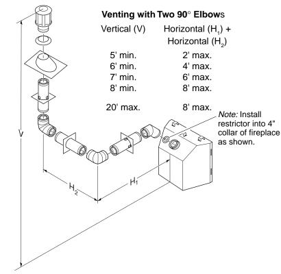
Figure 25 - Vertical Rigid Venting Configuration Using Two 90 $^\circ$  Elbows with Two Horizontal Runs
